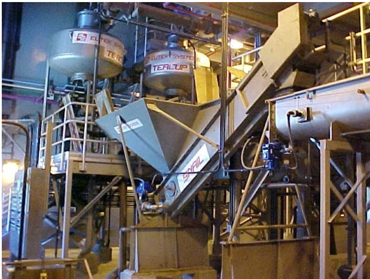
Figure 3 – Eutek TEACUP degritting system at MBC
